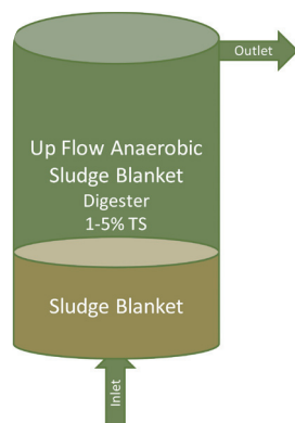
Upflow Sludge Blanket Anaerobic Digester (figure developed by Lucas Loetscher, Colorado State University)
